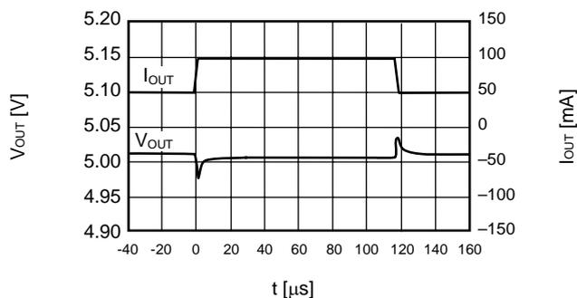
(3) Shutdown pin transient response characteristics
