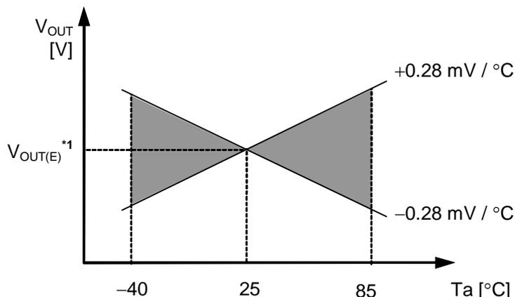
\*1.  $V_{OUT(E)}$  is the value of the output voltage measured at 25°C.
