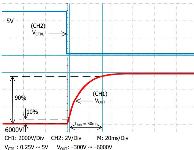
Figure 11. Falling Trail for Large Signal Response
