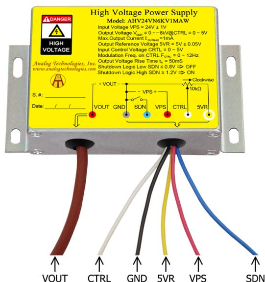
Figure 2. The Connecting Lead Wires of AHV24VN6KV1MA
