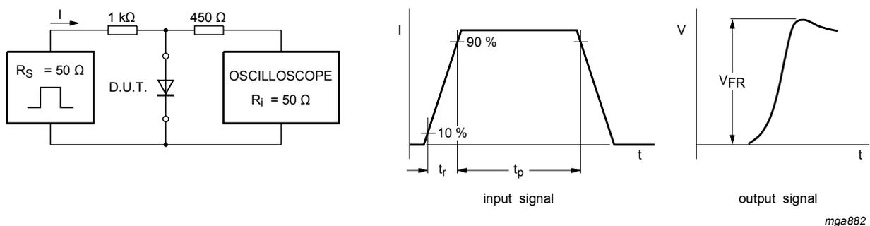
Fig. 10. Forward recovery voltage test circuit and waveforms
