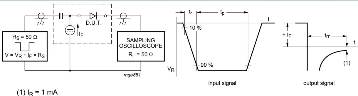
Fig. 9. Reverse recovery time test circuit and waveforms
