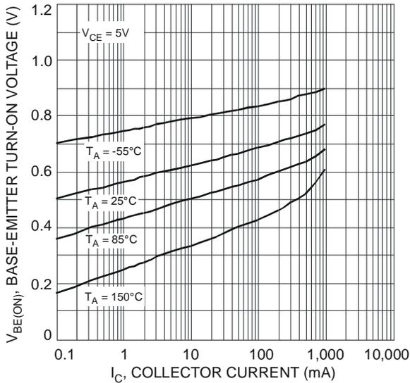
Fig. 7 Typical Base-Emitter Turn-On Voltage vs. Collector Current
