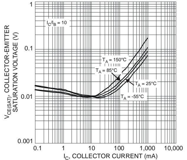
Fig. 6 Typical Collector-Emitter Saturation Voltage vs. Collector Current
