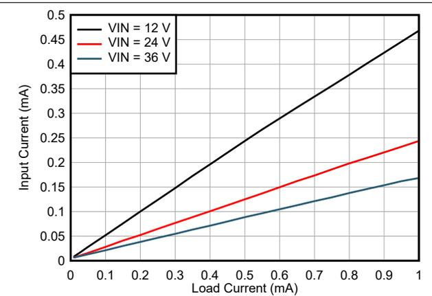
Figure 6-4. Input Current vs Load Current for 5 V<sub>OUT</sub>
