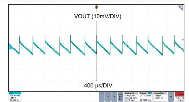
Figure 6-10. Output Ripple at 12 V<sub>IN</sub>, 5 V<sub>OUT</sub> (Fixed), 1 mA Load with 2 × 22 μF C<sub>OUT</sub>
