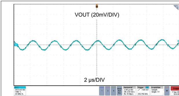
Figure 6-9. Output Ripple at 12 V<sub>IN</sub>, 5 V<sub>OUT</sub> (Fixed), 2-A Load with 2 × 22 μF C<sub>OUT</sub>
