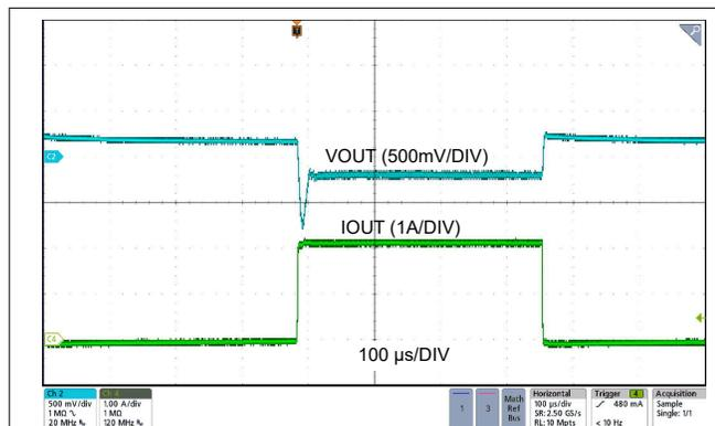
Figure 6-5. Load Transient 12 V<sub>IN</sub>, 5 V<sub>OUT</sub>, I<sub>OUT</sub> = 0 A to 2 A, Slew Rate = 1 A/μs (AUTO) with 2 × 22 μF C<sub>OUT</sub>
