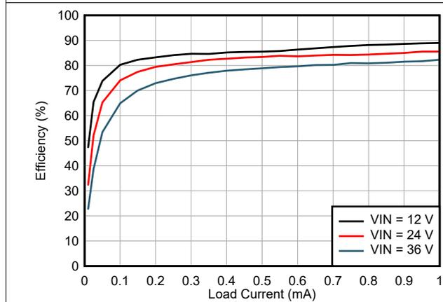
Figure 6-3. 5 V<sub>OUT</sub>, Light Load Efficiency
