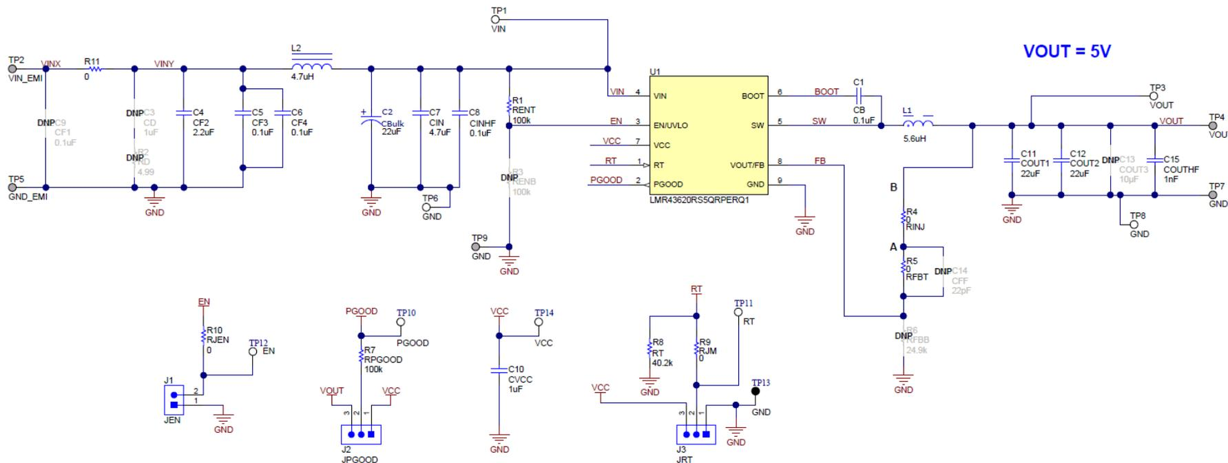
Figure 3-1. LMR43620RQ5EVM-400 Schematic
