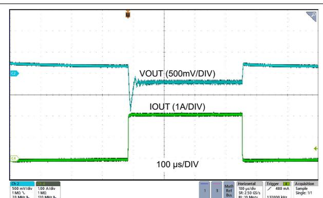
Figure 6-6. Load Transient 24 V<sub>IN</sub>, 5 V<sub>OUT</sub>, I<sub>OUT</sub> = 0 A to 2 A, Slew Rate = 1 A/μs (AUTO) with 2 × 22 μF C<sub>OUT</sub>
