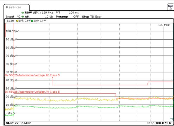
**Figure 6-13. LMR43620RQ5EVM-400 High Frequency Conducted EMI Results 12.5 V<sub>IN</sub>, 5 V<sub>OUT</sub>, I<sub>OUT</sub> = 2 A (Green-Average Scan and Yellow-Peak Scan)**
