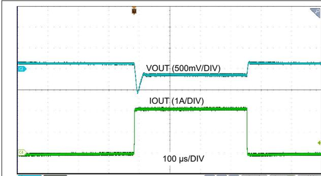
Figure 6-7. Load Transient 12 V<sub>IN</sub>, 5 V<sub>OUT</sub>, I<sub>OUT</sub> = 0 A to 2 A, Slew Rate = 1 A/μs (AUTO) with 3 × 22 μF C<sub>OUT</sub>
