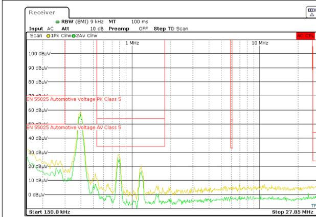
**Figure 6-12. LMR43620RQ5EVM-400 Low Frequency Conducted EMI Results 12.5 V<sub>IN</sub>, 5 V<sub>OUT</sub>, I<sub>OUT</sub> = 2 A (Green-Average Scan and Yellow-Peak Scan)**
