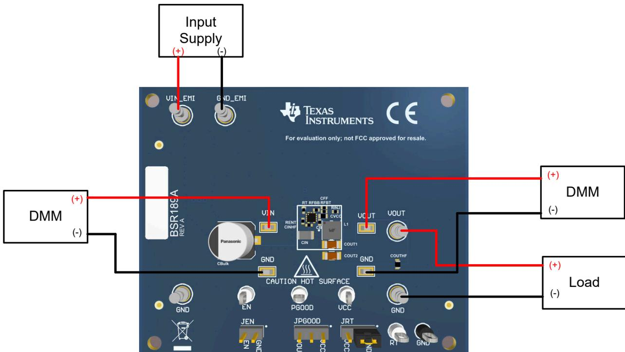
Figure 1-1. EVM Board Connections
