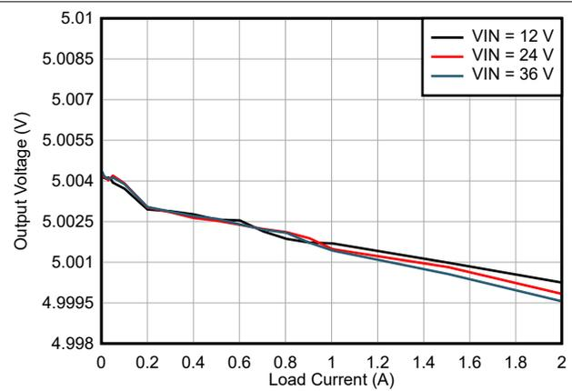
Figure 6-2. 5 V<sub>OUT</sub>, 400-kHz Load Regulation
