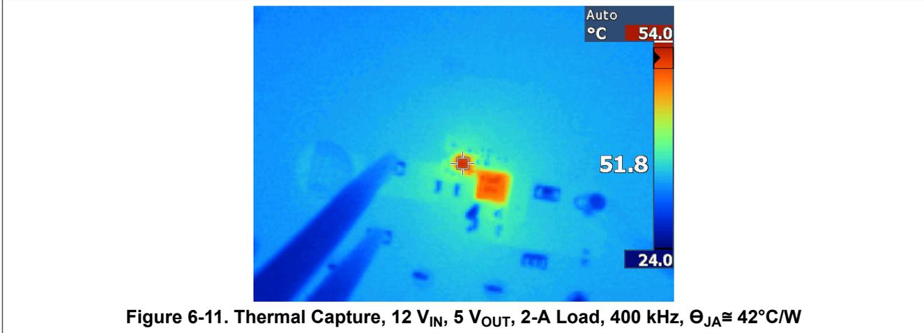
Figure 6-11. Thermal Capture, 12 V<sub>IN</sub>, 5 V<sub>OUT</sub>, 2-A Load, 400 kHz,  $\Theta_{JA} \approx 42^\circ\text{C/W}$
