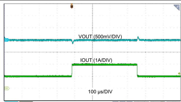
Figure 6-8. Load Transient 12 V<sub>IN</sub>, 5 V<sub>OUT</sub>, I<sub>OUT</sub> = 1 A to 2 A, Slew Rate = 1 A/μs (AUTO) with 3 × 22 μF C<sub>OUT</sub>
