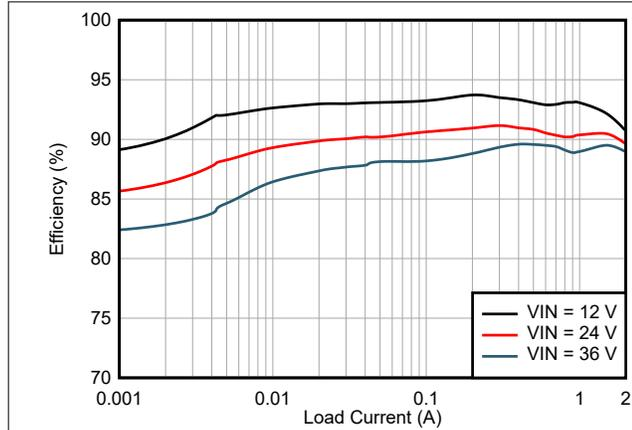
Figure 6-1. 5 V<sub>OUT</sub>, 400-kHz Efficiency
