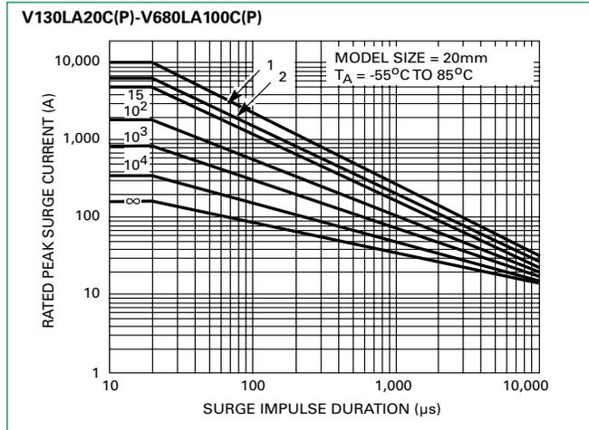
Note: Repetitive surge capability is qualified and tested based on 8/20us current waveform (not combination waveform) and UL1449 40.7.3 (Edition 4) test condition.
