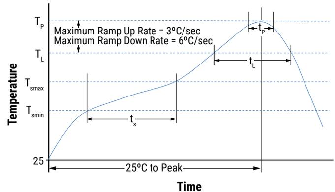
Note 1: All temperatures refer to the center of the package, measured on the capacitor body surface that is facing up during assembly reflow.
