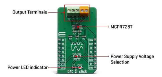
The MCP4728 device has a high precision internal voltage reference (VREF = 2.048V). The internal reference can be selected by user, or external reference may be used (VDD) for each channel individually. This gives the ADC 4 click good flexibility for use in various applications.
