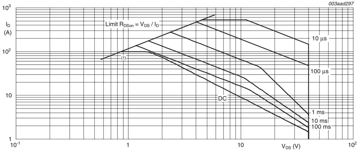
$T_{mb} = 25^\circ\text{C}; I_{DM}$  is single pulse
