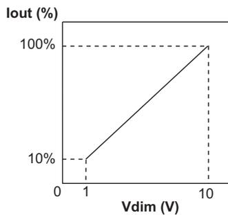
**PWM Dimming Curve**
