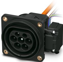
CHARX connect, Vehicle charging inlet, Locking actuator right, For charging electric vehicles (EV) with alternating current (AC), For installation in electric vehicles (EV), AC type 2, IEC 62196-2, length: 2 m, Locking actuator: 24 V, 4-position, M6, Generation 4, A protective cap is supplied as standard for the AC contacts.
