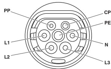
Pin assignment of Vehicle Inlet
