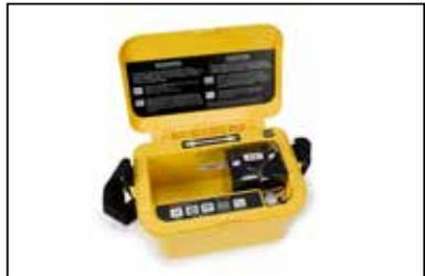
**Note:** *The internal batteries must be at least 5.4 volts. Do not remove the alkaline batteries from the transmitter when using the rechargeable battery. Rechargeable battery, or cigarette lighter adapter cable, is required for maximum output level. Rechargeable battery is shown installed in the well of the transmitter case.*
