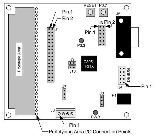
Figure 4. C8051F310 Target Board
