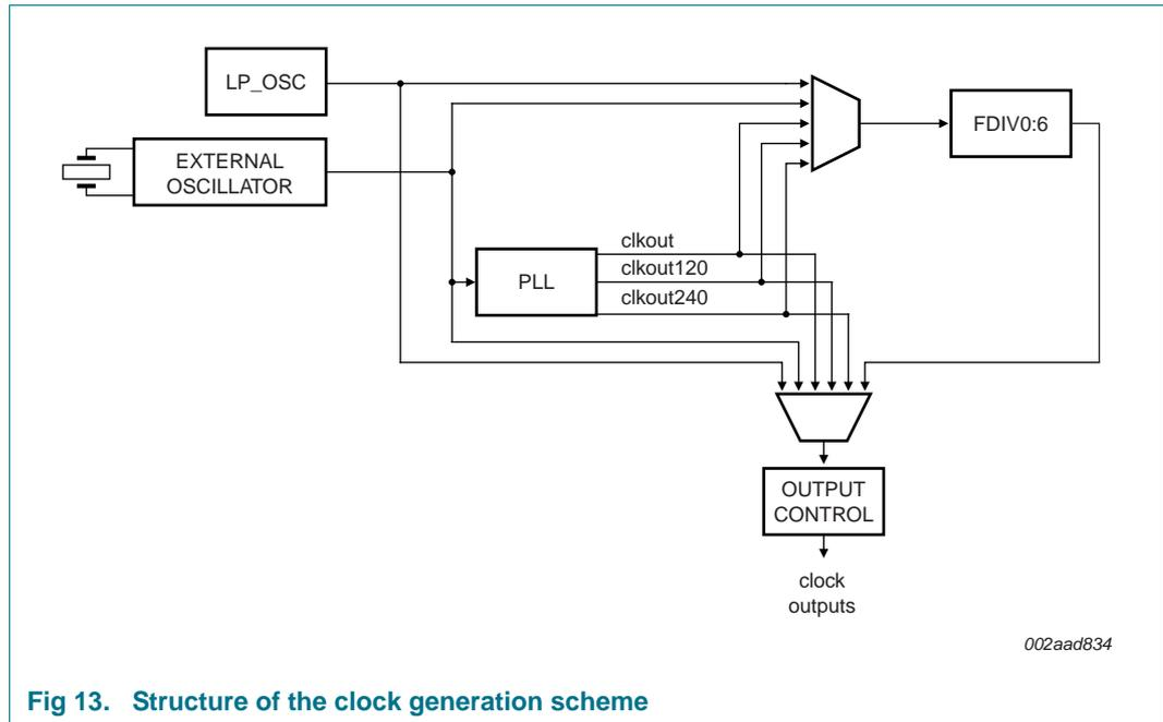
**Fig 13. Structure of the clock generation scheme**
