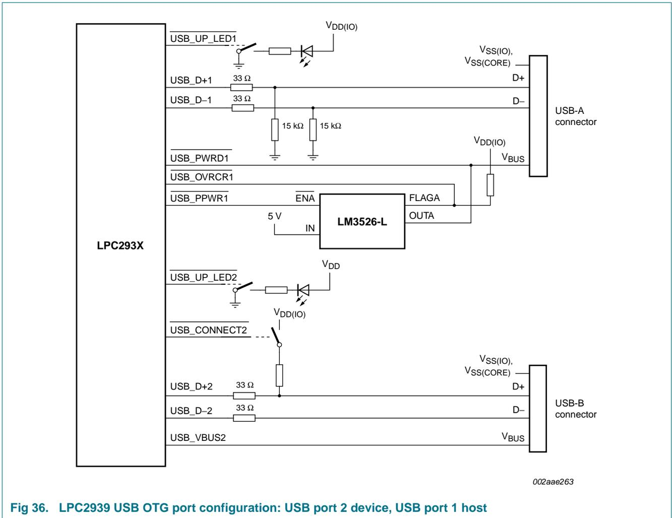
Fig 36. LPC2939 USB OTG port configuration: USB port 2 device, USB port 1 host
