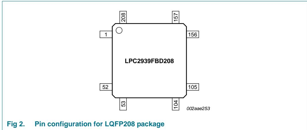
Fig 2. Pin configuration for LQFP208 package
