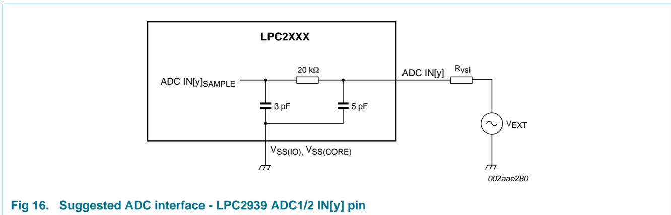
**Fig 16. Suggested ADC interface - LPC2939 ADC1/2 IN[y] pin**
