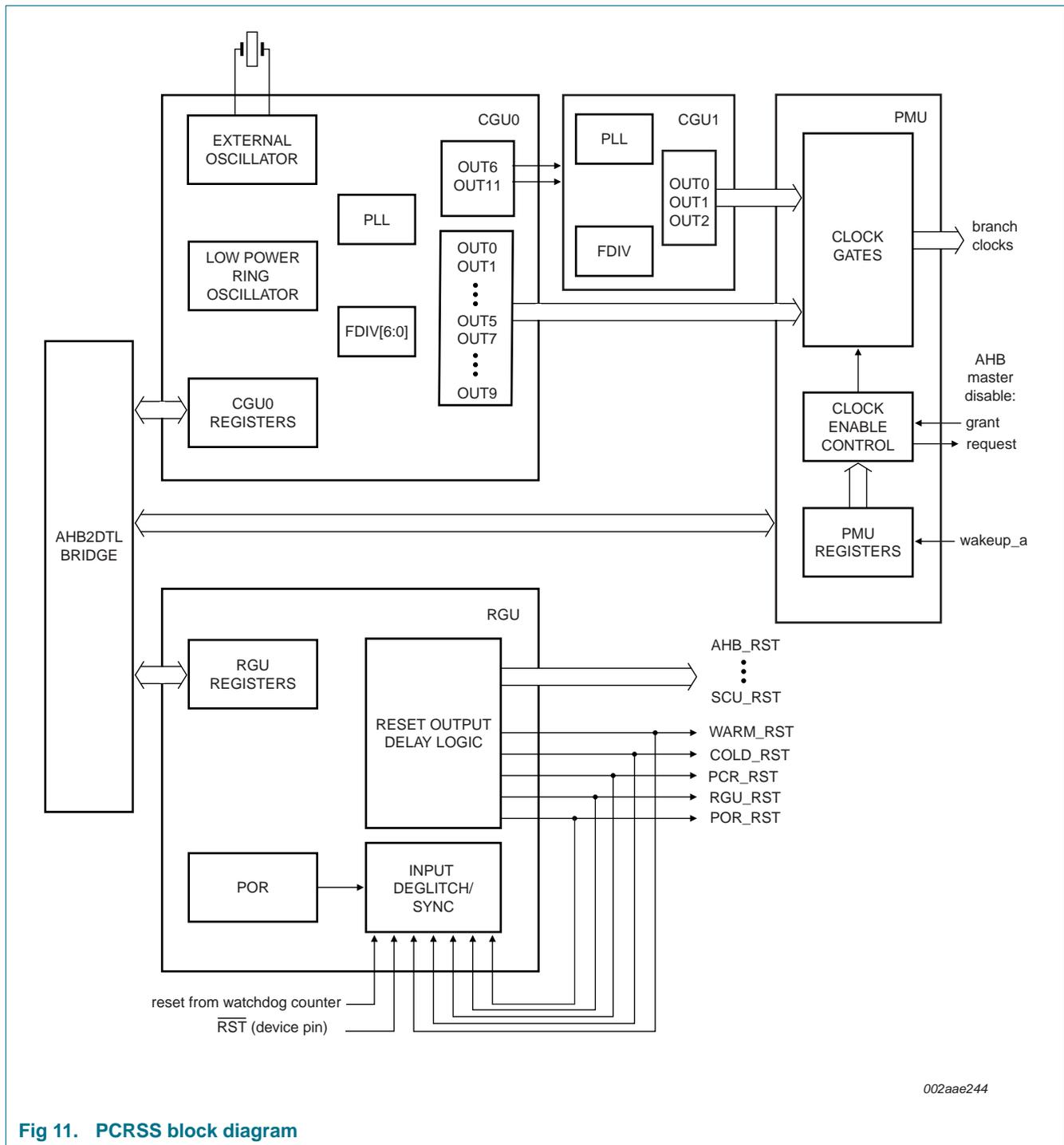
Fig 11. PCRSS block diagram
