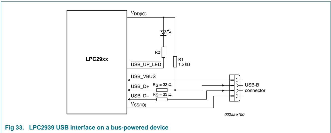
Fig 33. LPC2939 USB interface on a bus-powered device
