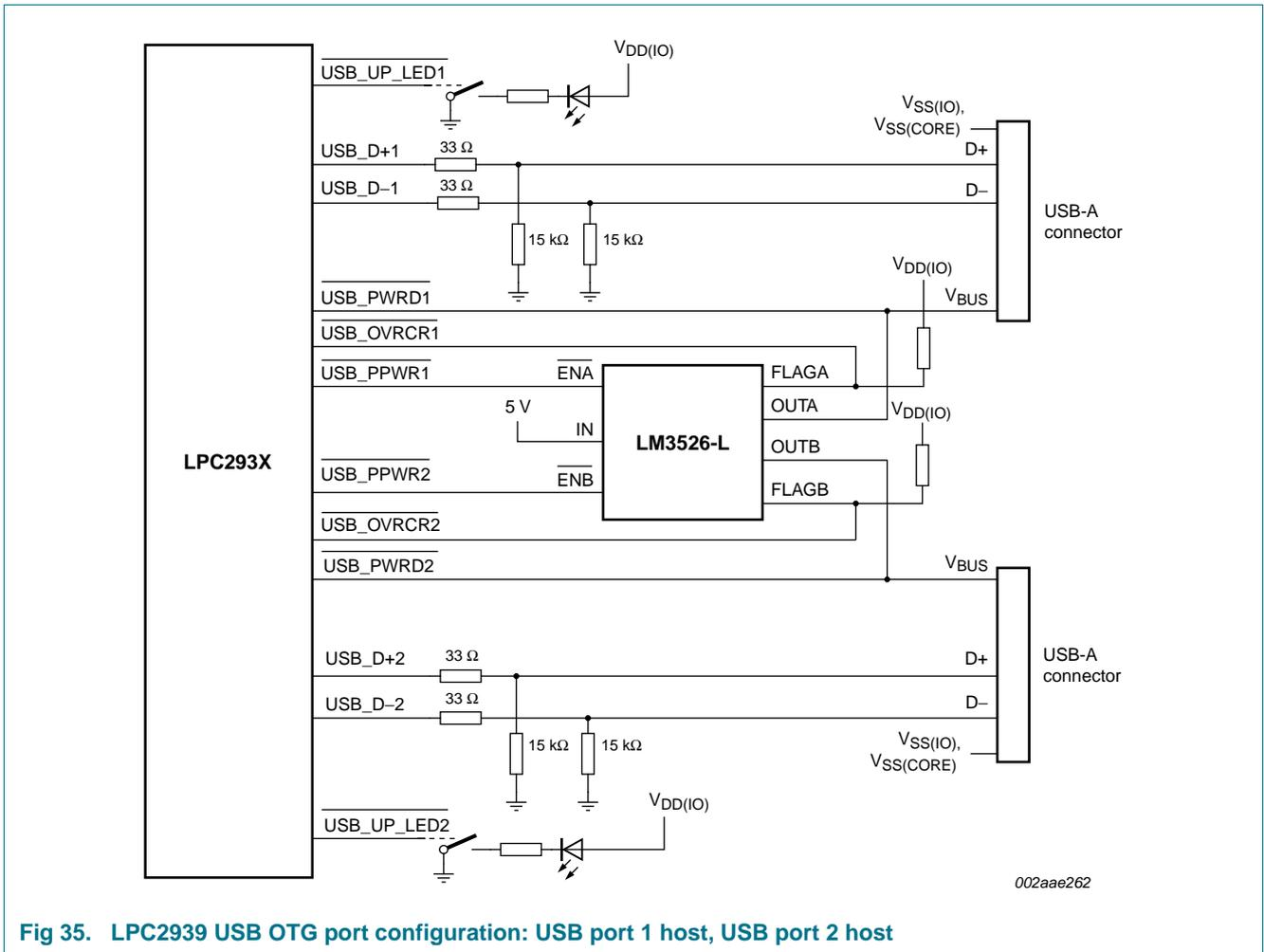
Fig 35. LPC2939 USB OTG port configuration: USB port 1 host, USB port 2 host
