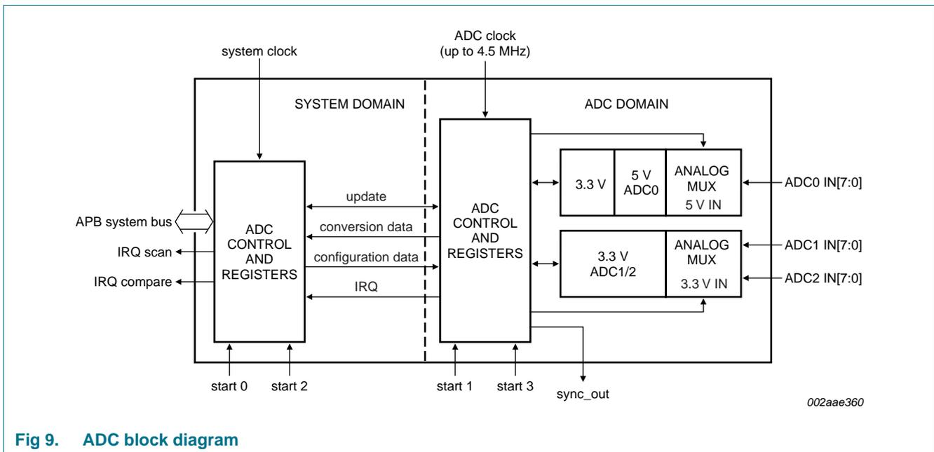
Fig 9. ADC block diagram
