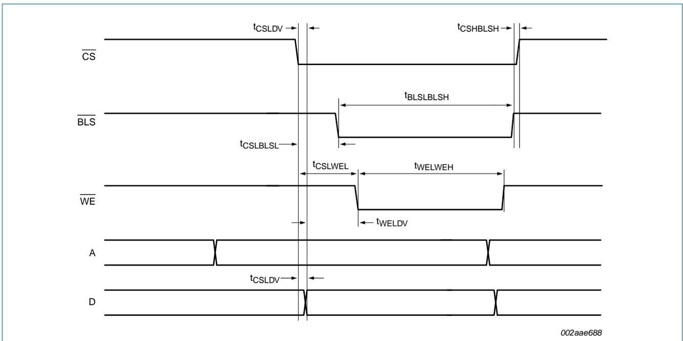
Fig 29. External memory write access
