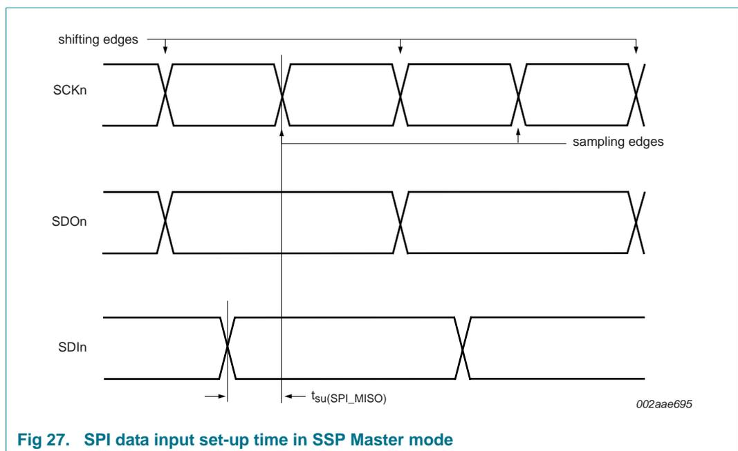
**Fig 27. SPI data input set-up time in SSP Master mode**
