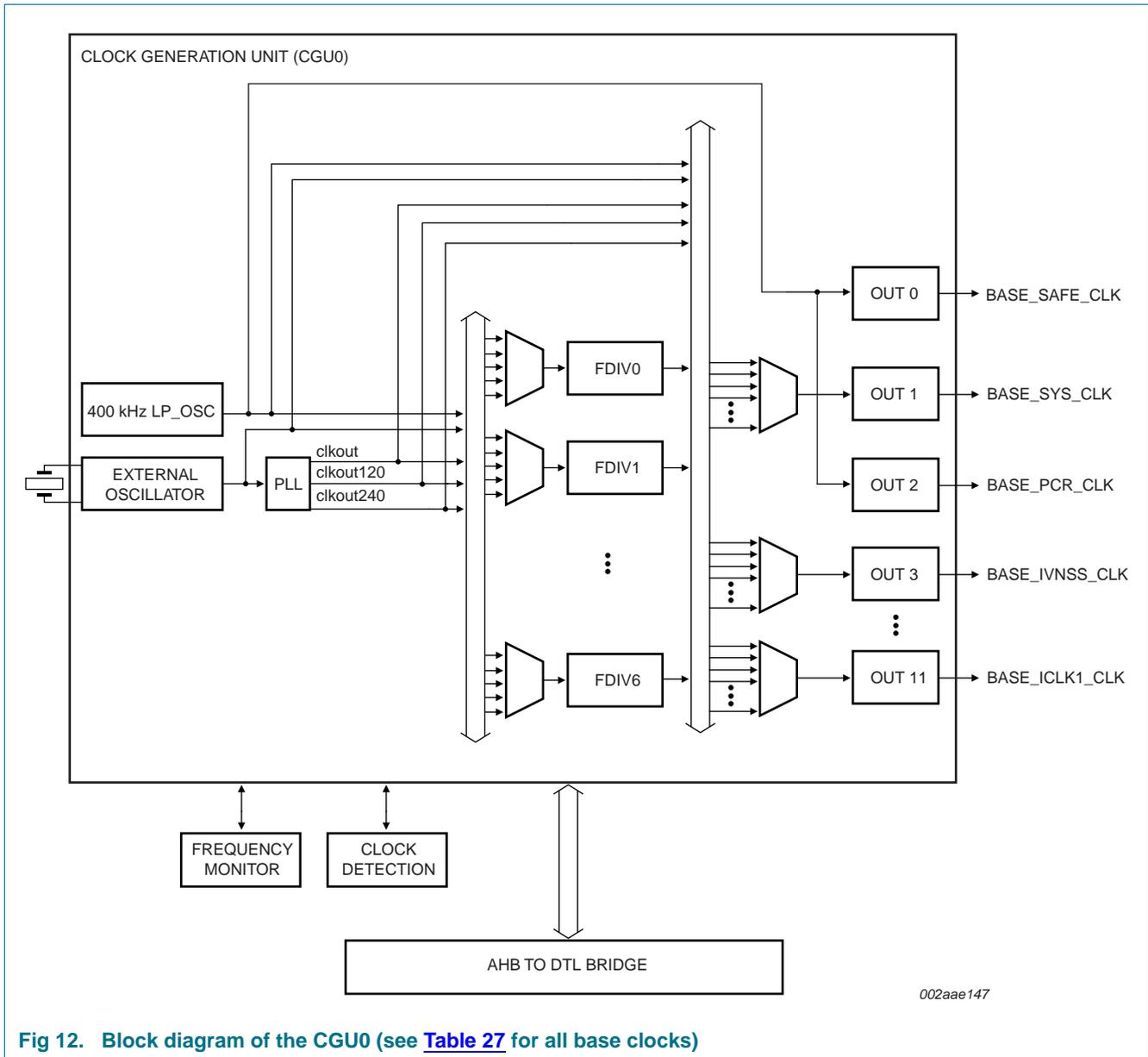
Fig 12. Block diagram of the CGU0 (see Table 27 for all base clocks)
