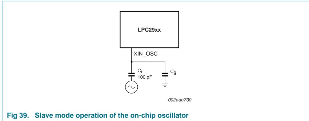
Fig 39. Slave mode operation of the on-chip oscillator
