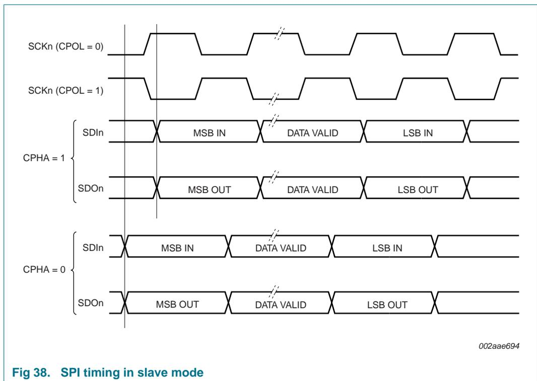
Fig 38. SPI timing in slave mode
