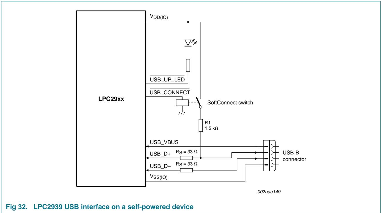
Fig 32. LPC2939 USB interface on a self-powered device
