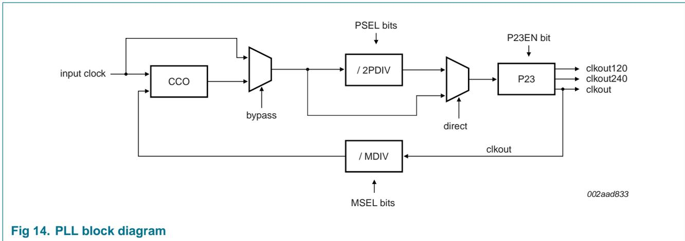
Fig 14. PLL block diagram
