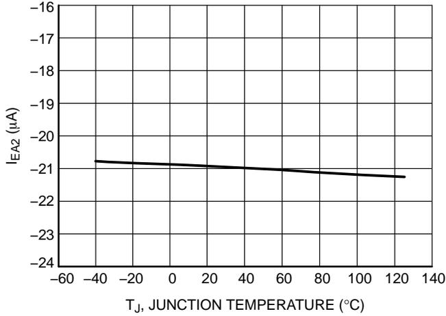
Figure 17. Error Amplifier Current Capability, Sinking (I<sub>EA2</sub>) vs. Junction Temperature
