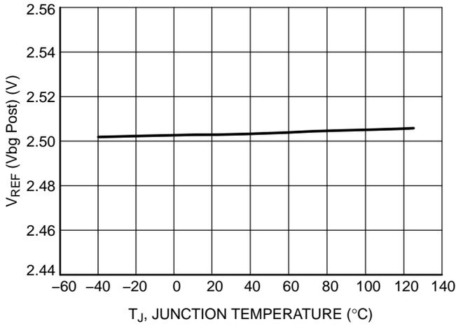
Figure 15. Feedback Voltage Reference (V<sub>REF</sub>) vs. Junction Temperature
