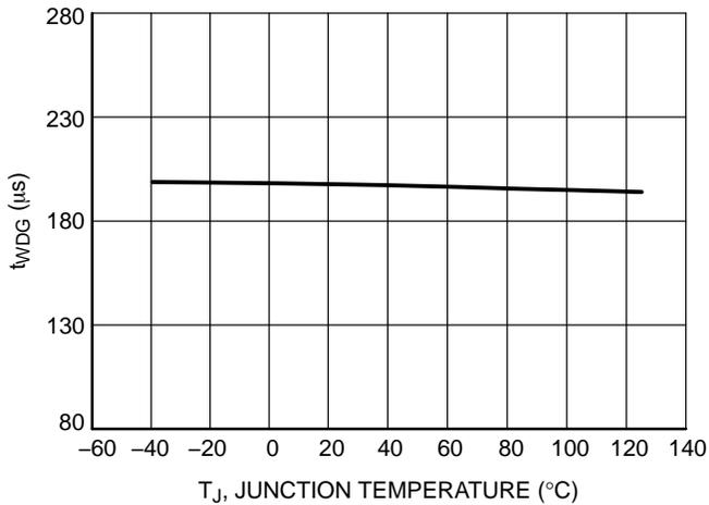
Figure 19. Watch Dog Timer Duration (t<sub>WDG</sub>) vs. Junction Temperature
