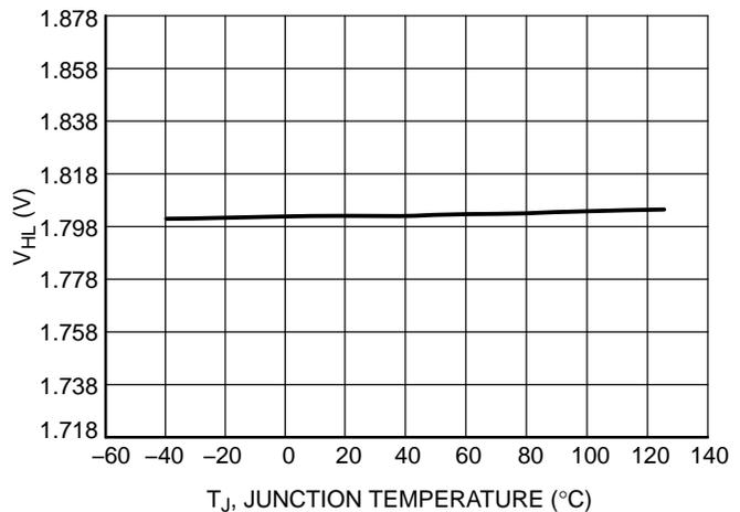
**Figure 26. Comparator Threshold for Line Range Detection, avg(V<sub>CS</sub>) Rising, (V<sub>HL</sub>) vs. Junction Temperature**
