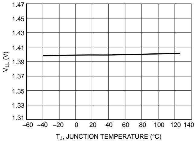
**Figure 27. Comparator Threshold for Line Range Detection, avg(V<sub>CS</sub>) Falling, (V<sub>LL</sub>) vs. Junction Temperature**
