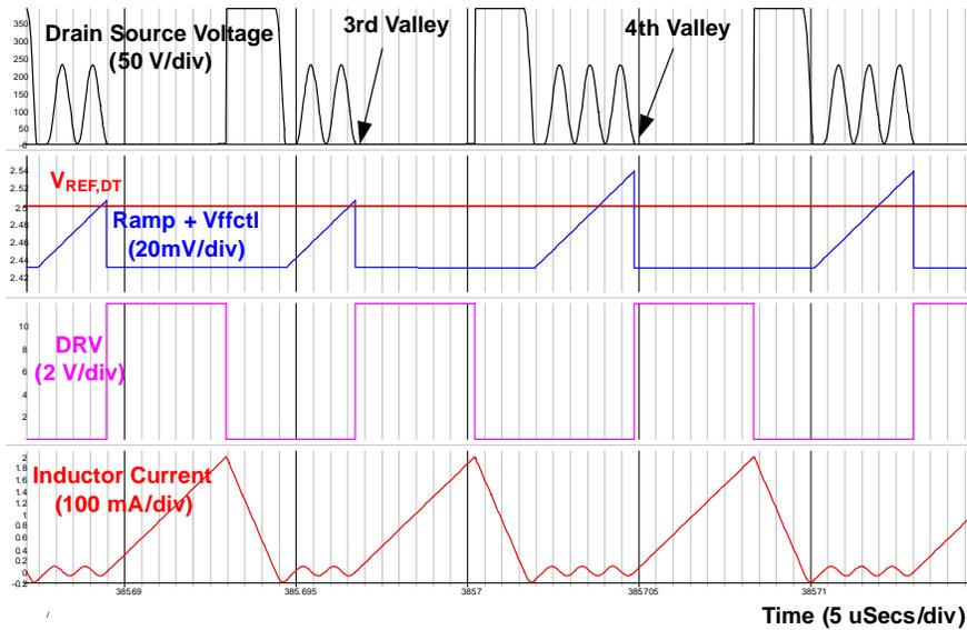
Figure 31. Clean Transition Without Hesitation Between Valleys
