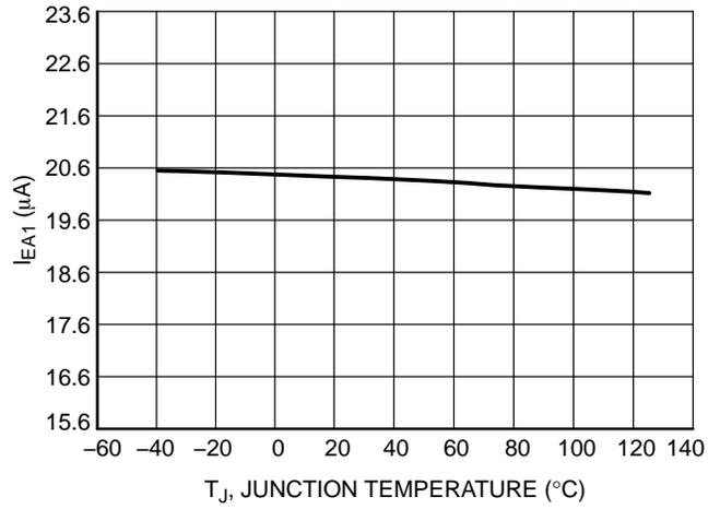
Figure 16. Error Amplifier Current Capability, Sourcing (I<sub>EA1</sub>) vs. Junction Temperature
