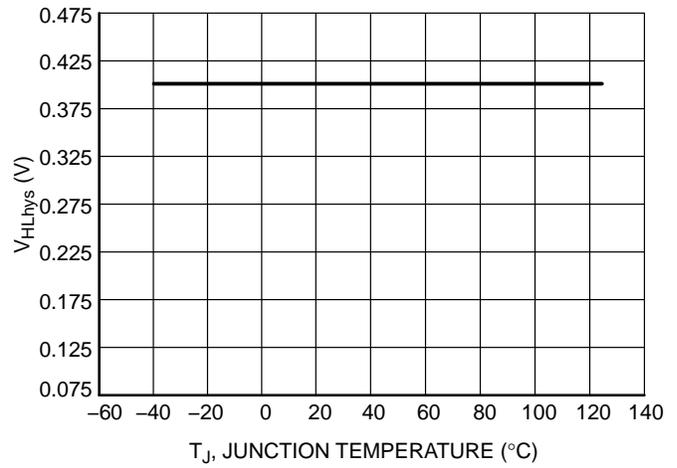
**Figure 28. Comparator Hysteresis for Line Range Detection, (V<sub>HL(hyst)</sub>) vs. Junction Temperature**
