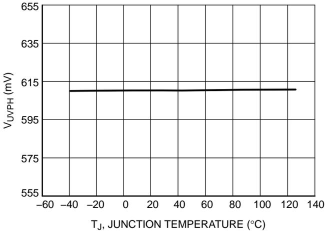
**Figure 23. UVP Threshold, V<sub>FB</sub> Increasing (V<sub>UVPH</sub>) vs. Junction Temperature**
