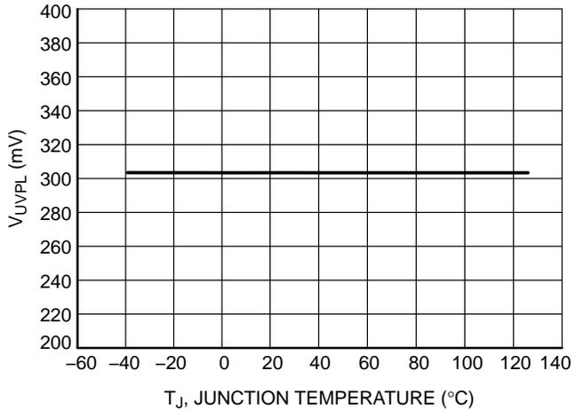
**Figure 24. UVP Threshold, V<sub>FB</sub> Decreasing (V<sub>UVPL</sub>) vs. Junction Temperature**
