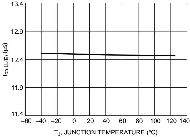
**Figure 21. Maximum On Time, avg(V<sub>CS</sub>) = 0.9 V & V<sub>ctrl</sub> Maximum (CrM) & Low Line for E Version (t<sub>on,LL,E</sub>) vs. Junction Temperature**
