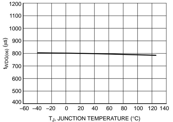
Figure 20. Watch Dog Timer Duration in "OverStress" Situation (t<sub>WDG(OS)</sub>) vs. Junction Temperature
