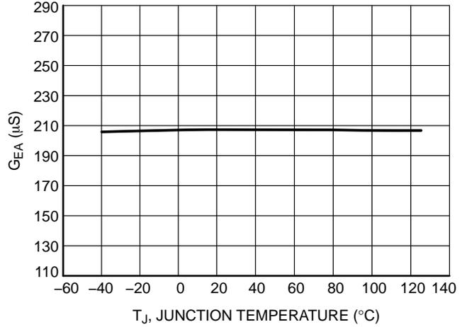
Figure 18. Error Amplifier Transconductance (G<sub>EA</sub>) vs. Junction Temperature
