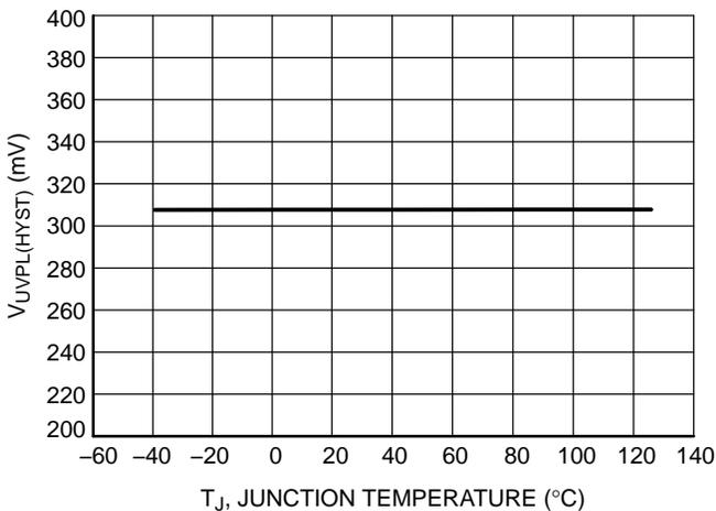
**Figure 25. UVP Threshold Hysteresis (V<sub>UVPL(HYST)</sub>) vs. Junction Temperature**
