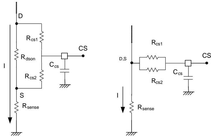
Figure 36. Current Sensing during the  $T_{ON}$  Phase
