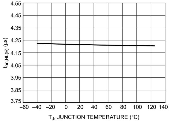
**Figure 22. Maximum On Time, avg(V<sub>CS</sub>) = 2.8 V & V<sub>ctrl</sub> Maximum (CrM) & High Line for E Version (t<sub>on,HL,E</sub>) vs. Junction Temperature**
