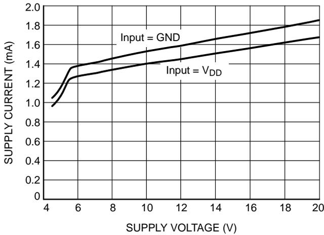
Figure 14. Supply Current vs. Supply Voltage (NCP81071B)
