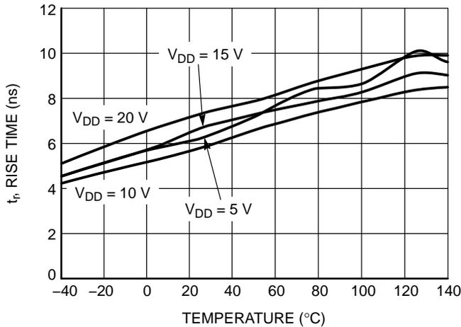
Figure 16. Rise Time vs. Temperature
