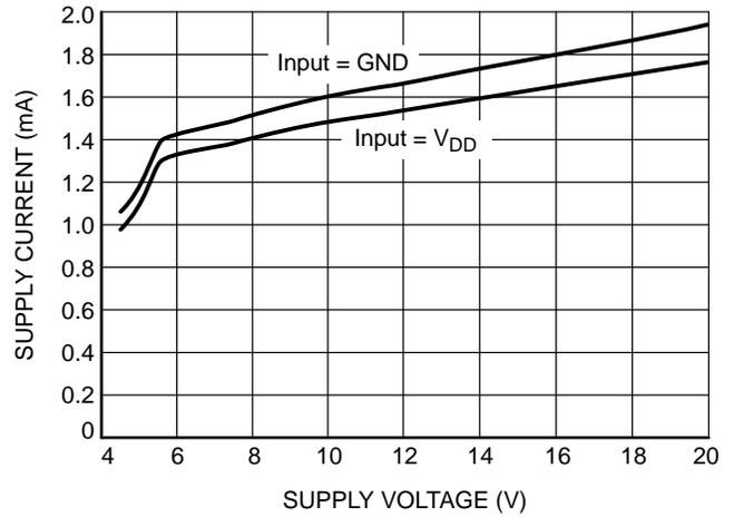
Figure 13. Supply Current vs. Supply Voltage (NCP81071A)
