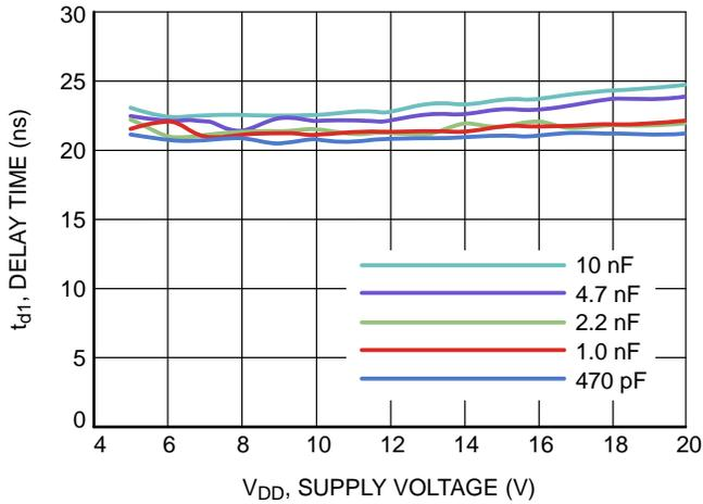
Figure 18. Propagation Delay  $t_{d1}$  vs. Supply Voltage
