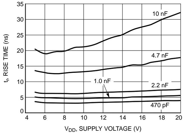
Figure 21. Rise Time  $t_r$  vs. Supply Voltage
