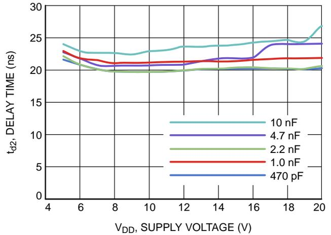
Figure 19. Propagation Delay  $t_{d2}$  vs. Supply Voltage
