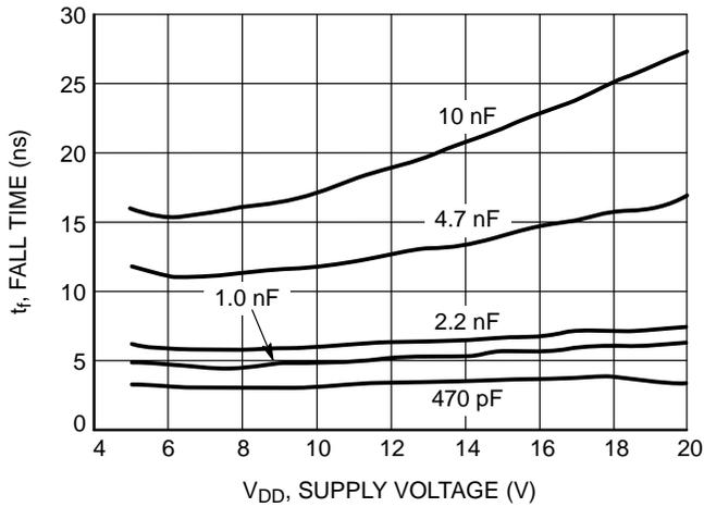
Figure 20. Fall Time  $t_f$  vs. Supply Voltage
