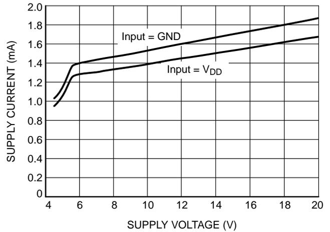
Figure 15. Supply Current vs. Supply Voltage (NCP81071C)
