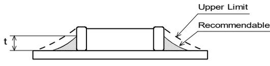
Accordingly increasing the solder volume, the mechanical stress to product is also increased. Exceeding solder volume may cause the failure of mechanical or electrical performance.
