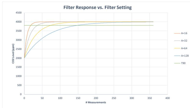
The graph above shows the effect of the filter on response times. Increasing the filter setting increases the measurement output response time. T<sub>90</sub> is the time to 90% of reading. The CozIR<sup>®</sup>-A takes 2 readings per second.
