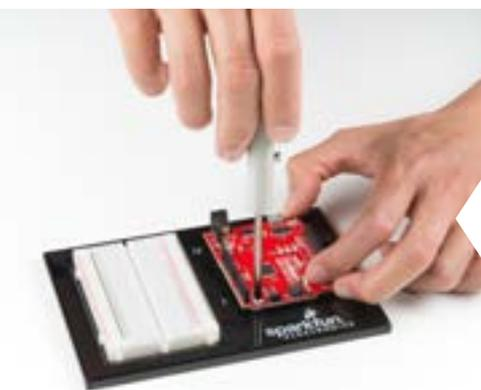
**ALIGN THE REDBOARD** with its spot on the baseplate. The text on it should face the same direction as the text on the breadboard and the baseplate. Using one of the two included screws, affix the RedBoard to one of the four stand-off holes found on the baseplate. The plastic holes are not threaded, so you will need to apply pressure as you twist the screwdriver.
