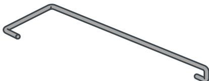
**3.** Attach the hook end of the linkage rod to the end hole on your servo mount. The motor should be reattached to the baseplate with Dual Lock.
