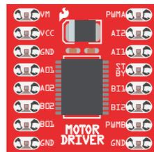
contain a set of switches (called an H-bridge) that lets you easily control the direction of one or more motors. The
