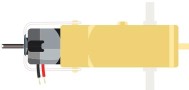
have a clever design allowing you to attach things that you want to spin fast (like a small fan or flag) to the hobby motor, and things that you want to be strong (like a wheel) to the plastic axle sticking out the
