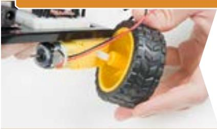
**5. ATTACH THE WHEELS** by sliding them onto the plastic shafts on the gearmotor. The shaft is flat on one side, as is the wheel coupler. Align the two, and then press to fit the wheel onto the shaft.
