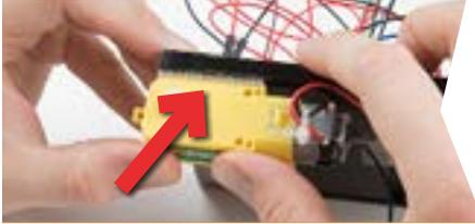
**3. PRESS THE MOTORS TO THE BASEPLATE**, connecting the two Dual Lock surfaces. Try to get the motors as straight as possible so your robot will drive straight.
