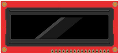
a potentiometer, the contrast can be adjusted. As you rotate the knob on the potentiometer, you should notice that the screen will get brighter or darker and that the characters become more visible or less visible. The contrast of LCDs is highly dependent on factors such as temperature and the voltage used to power them. Thus, external contrast knobs are needed for displays that cannot automatically account for temperature and voltage changes.
