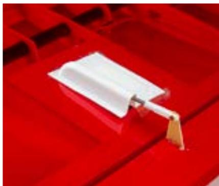
Linkage rods are found on many RC airplanes, which use servo motors to control the ailerons, elevators and rudder.
