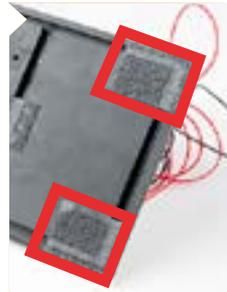
**2. CUT TWO MORE STRIPS** that are 1.25 inches (3.175cm) long and  $\frac{3}{4}$  inch (1.9cm) wide. Remove the adhesive backing, and attach the strips to the two motors. Be sure that your motors are mirror images of each other when you attach the Dual Lock.
