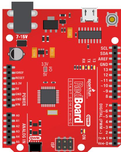
**THE SPARKFUN REDBOARD QWIIIC** is one of a multitude of development boards based on the ATmega328 microprocessor. It has 14 digital input/output pins (six of which can be PWM outputs), six analog inputs, a 16MHz crystal oscillator, a USB connection, a power jack, and a reset button. You’ll learn more about each of the RedBoard’s features as you progress through this guide.
