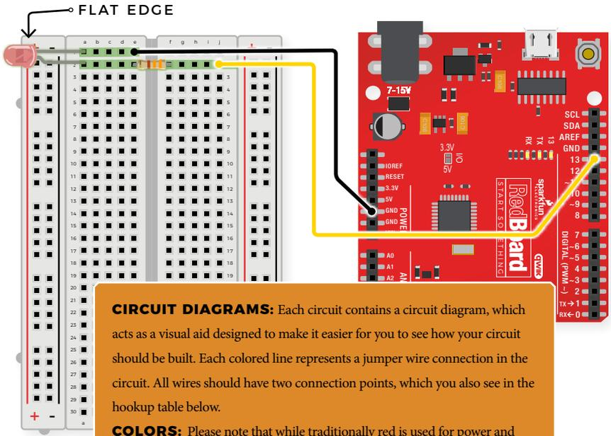
**CIRCUIT DIAGRAMS:** Each circuit contains a circuit diagram, which acts as a visual aid designed to make it easier for you to see how your circuit should be built. Each colored line represents a jumper wire connection in the circuit. All wires should have two connection points, which you also see in the hookup table below.
