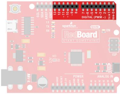
**DIGITAL OUTPUT:** When working with microcontrollers such as the RedBoard, there are a variety of pins to which you can connect electronic components. Knowing which pins perform which functions is important when building your circuit. In this circuit, we will be using what is known as a digital output. There are 14 of these pins found on the RedBoard.
