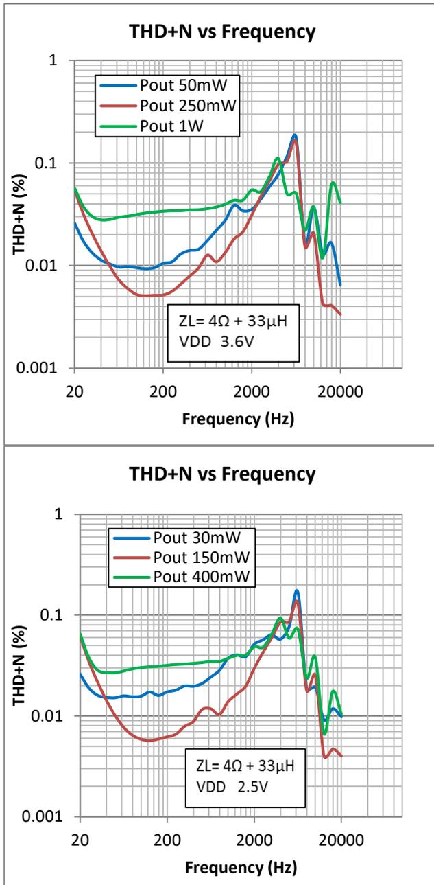
**Note: All the above plots are captured with 0.1uF input capacitor. It is recommended to use 2.2uF input capacitor to get a flat low frequency response.**
