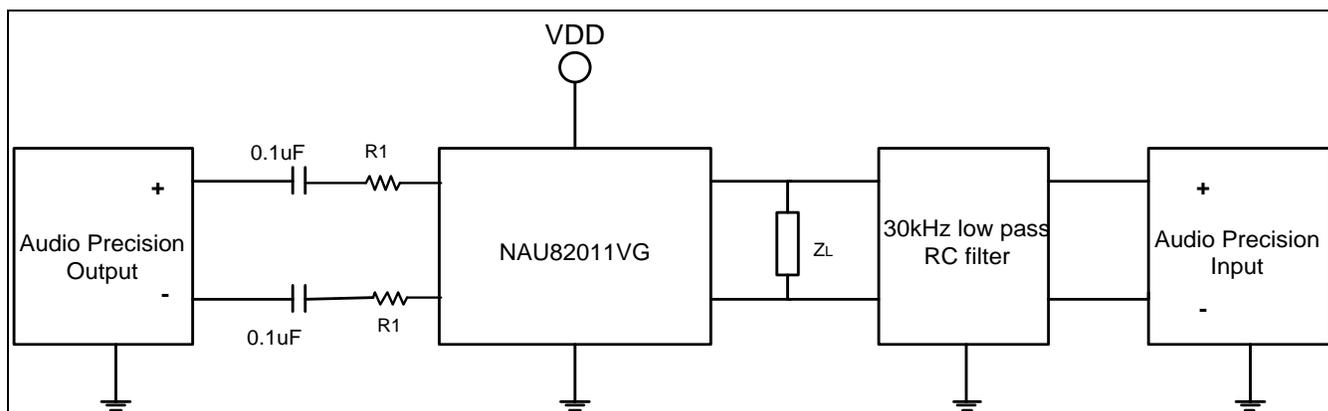
**Note:** The 30kHz low pass RC filter is implemented by using R= 1k Ohm and C = 4.7nF
