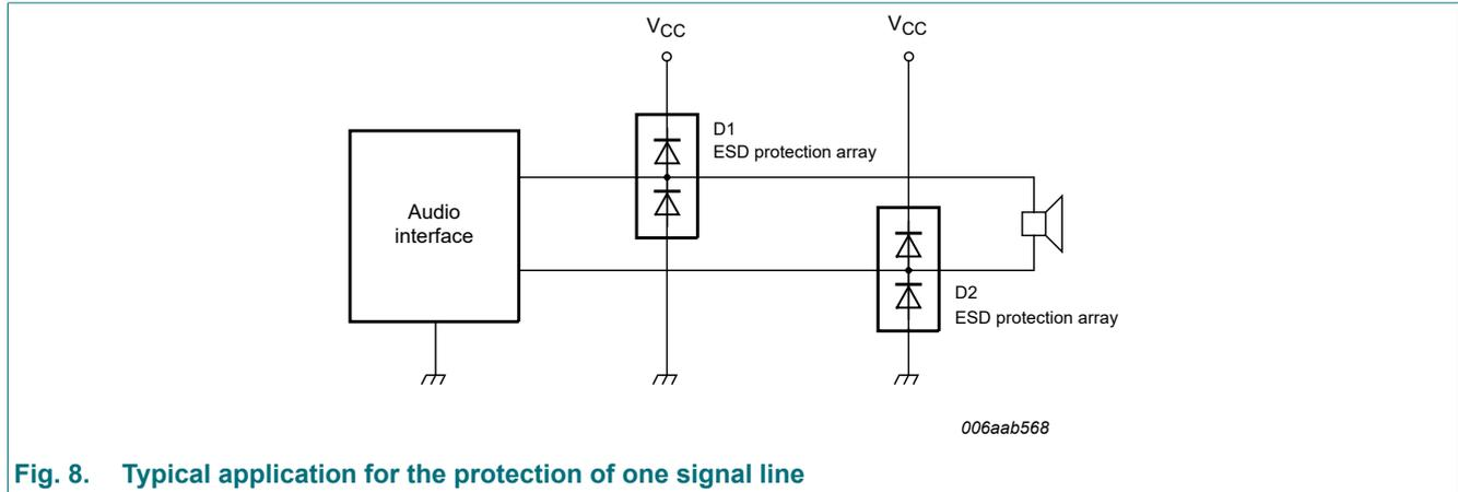
Fig. 8. Typical application for the protection of one signal line
