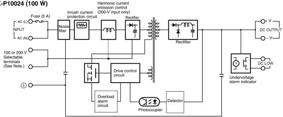
Note: Use the short bar to short-circuit terminals 7 and 8 to select 100 to 120 VAC and remove the short bar to select 200 to 240 VAC.
