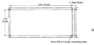
Note: If more than one Power Supply is installed in a row, keep a distance of 20 mm min. (L = 20 mm min.) between each adjacent Power Supply.
