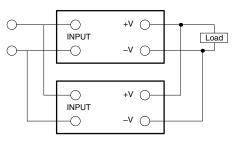
Note: When operating the S82K-P10024 or 240-W model in parallel operation, set the switch to "PARALLEL." Refer to the derating curve for the rated current under this operation.
