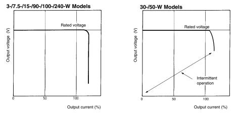
Note: Do not short-circuit the output terminals of the S82K or use the S82K with excessive output current for a long time, otherwise the internal circuitry of the S82K may be deteriorated or damaged.
