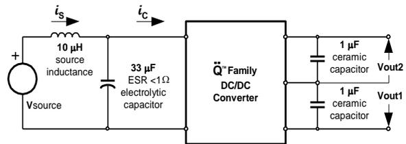
Figure 34. Test setup for measuring input reflected ripple currents, Ic and Is.
