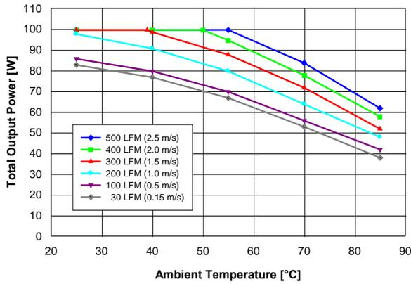
Figure 11. Available output power for balanced load current ( $I_{out1} = 1.5 \cdot I_{out2}$ ) vs. ambient air temperature and airflow rates for converter mounted vertically with  $V_{in} = 48\text{ V}$ , air flowing from pin 3 to pin 4 and maximum FET temperature  $\leq 120\text{ }^\circ\text{C}$ .
