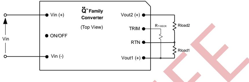
Figure 3. Configuration for decreasing output voltage.
