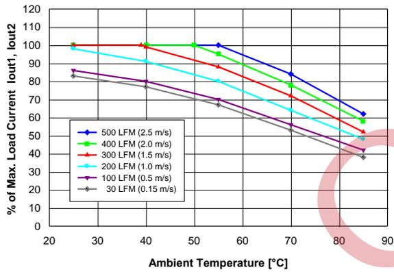
Figure 13. Available balanced load current ( $I_{out1} = 1.5 \cdot I_{out2}$ ) vs. ambient air temperature and airflow rates for converter mounted vertical-ly with  $V_{in} = 48\text{ V}$ , air flowing from pin 3 to pin 4 and maximum FET temperature  $\leq 120\text{ }^\circ\text{C}$ .
