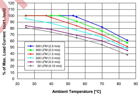
Figure 10. Available balanced load current ( $l_{out1} = 1.5 \cdot l_{out2}$ ) vs. ambient temperature and airflow rates for converter mounted horizontally with  $V_{in} = 48 V$ , air flowing from pin 3 to pin 4 and maximum FET temperature  $\leq 120\text{ }^{\circ}C$ .
