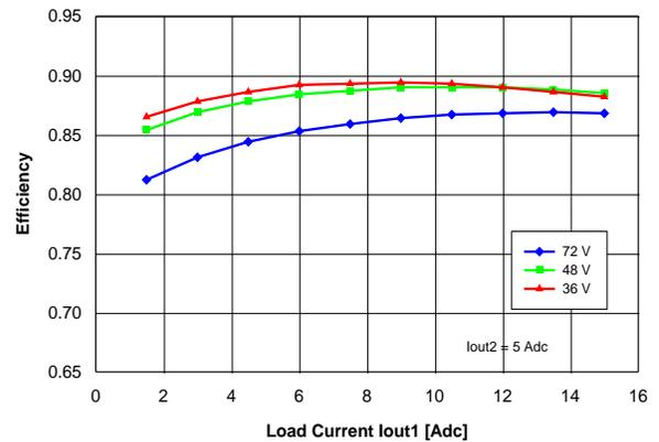
Figure 16. Efficiency vs. load current  $I_{out1}$  and input voltage for converter mounted horizontally with air flowing from pin 3 to pin 4 at a rate of 300 LFM (1.5 m/s), for  $I_{out2} = 5\text{ A}$  and  $T_a = 25\text{ }^\circ\text{C}$ .
