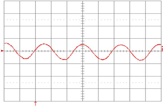
Figure 35. Input reflected ripple current,  $I_r$  (100 mA/div), measured at input terminals at full rated load current on both outputs and  $V_{in} = 48$  V. Refer to Fig. 34 for test setup. Time scale: 1  $\mu$ s/div.
