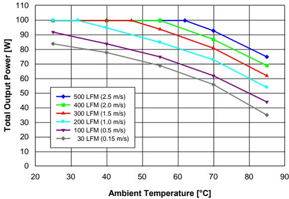
Figure 7. Available output power for balanced load current ( $l_{out1} = 1.5 \cdot l_{out2}$ ) vs. ambient air temperature and airflow rates for converter mounted vertically with  $V_{in} = 48 V$ , air flowing from pin 3 to pin 1 and maximum FET temperature  $\leq 120\text{ }^{\circ}C$ .
