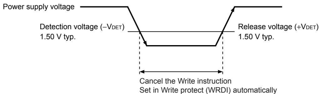
**Figure 18** Operation during Low Power Supply Voltage
