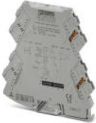
Configurable temperature transducer with plug-in connection technology for connecting thermocouples. Configurable via DIP switch or software. Push-in connection technology, standard configuration
