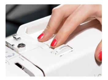
You may need to adjust the tension on your machine. Experiment on a scrap piece of fabric and examine the balance between the conductive and regular thread. Adjust the tension and experiment again until you are satisfied.
