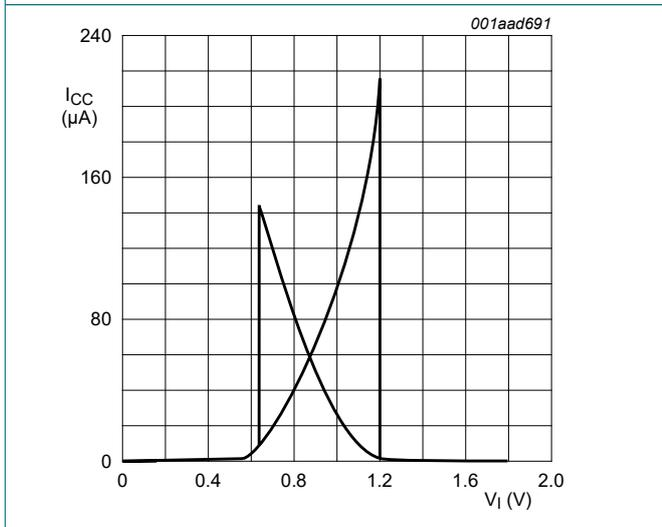
Fig. 15. Typical transfer characteristics; V<sub>CC</sub> = 1.8 V
