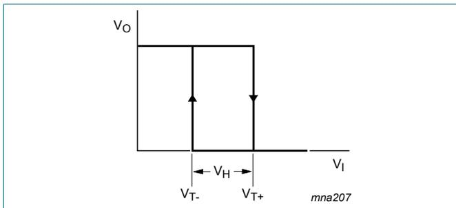
Fig. 13. Transfer characteristic
