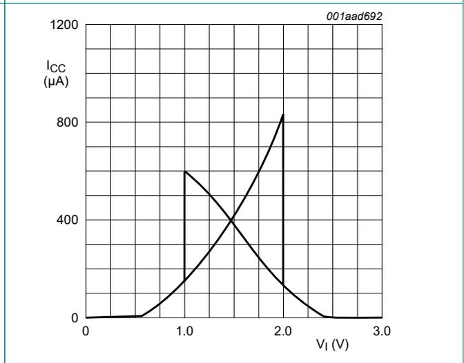
Fig. 16. Typical transfer characteristics; V<sub>CC</sub> = 3.0 V
