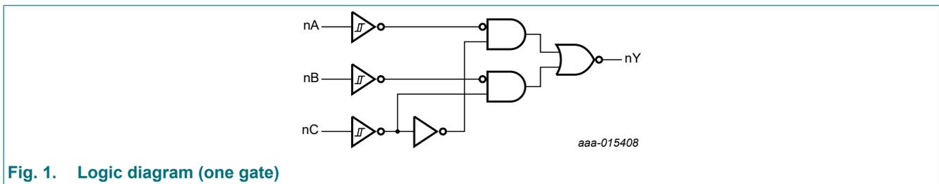
Fig. 1. Logic diagram (one gate)
