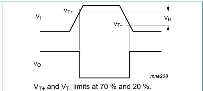
Fig. 14. Definition of V<sub>T+</sub>, V<sub>T-</sub> and V<sub>H</sub>
