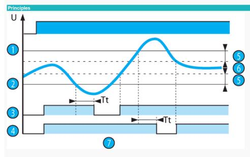
If the frequency of the controlled voltage exceeds the preset overfrequency threshold for longer than the time set on the front face (0.1 to 10 s), the corresponding output relay opens and its LED is extinguished. During the time delay, this LED flashes.
