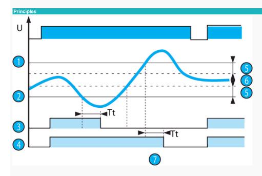
If "with memory" mode has been selected, the relay opens and stays in this position when threshold crossing is detected. The power supply must be disconnected to reset the product.
