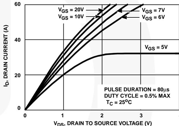
FIGURE 8. SATURATION CHARACTERISTICS
