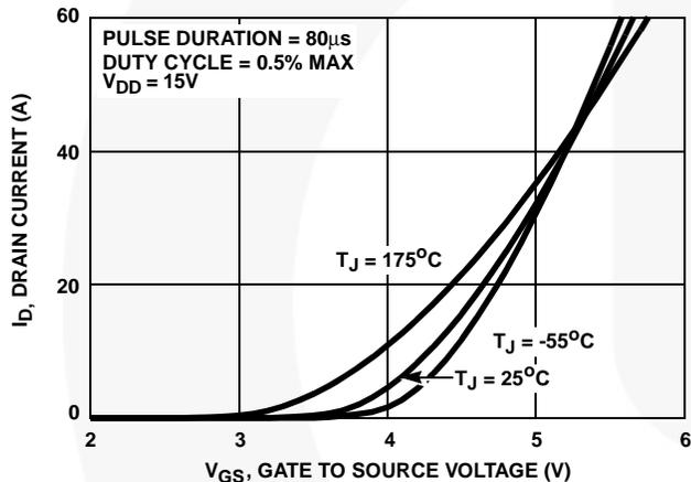
FIGURE 7. TRANSFER CHARACTERISTICS
