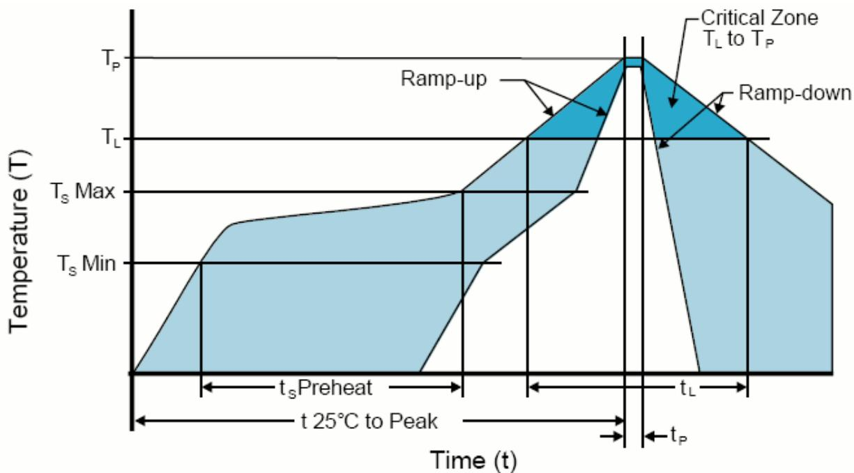
**LOW TEMPERATURE INFRARED/CONVECTION**
