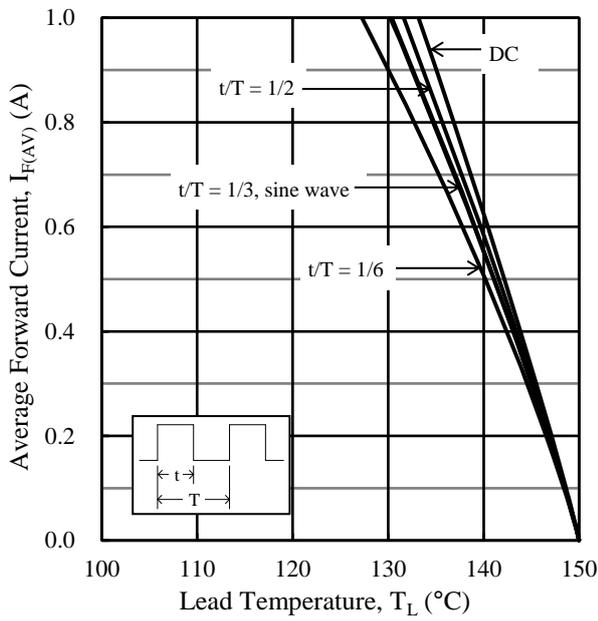
Figure 2.  $I_{F(AV)}$  vs.  $T_L$  <sup>(2)</sup> ( $T_J = 150$  °C,  $V_R = 0$  V)
