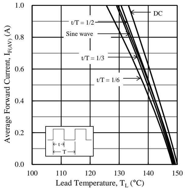
Figure 3.  $I_{F(AV)}$  vs.  $T_L$  <sup>(2)</sup> ( $T_J = 150$  °C,  $V_R = 200$  V)
