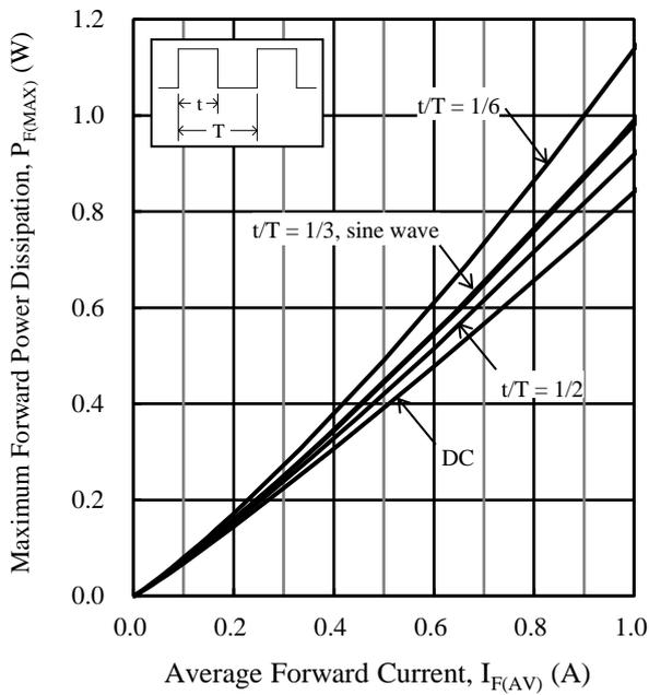
Figure 4.  $P_{F(MAX)}$  vs.  $I_{F(AV)}$  ( $T_J = 150\text{ }^\circ\text{C}$ )
