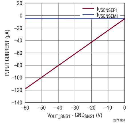
**+1.8V Channel Voltage Sense Input Currents vs Differential Input Voltage**
