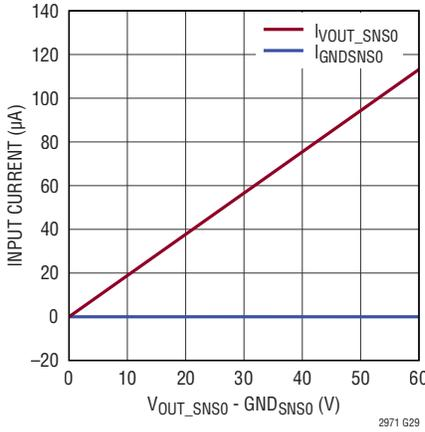
**-60V Channel Voltage Sense Input Currents vs Differential Input Voltage**
