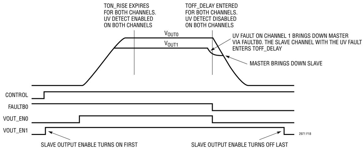
**Figure 18. Fault on Channel 1 Tracking All Supplies Down**
