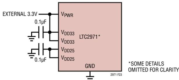
Figure 23. Powering LTC2971 from External 3.3V Supply
