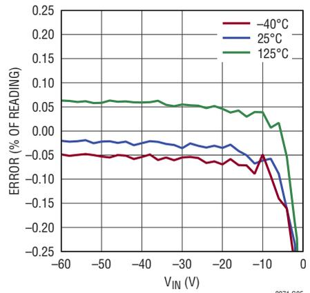
**+1.8V Channel READ\_VOUT Total Unadjusted Error vs Input Voltage**
