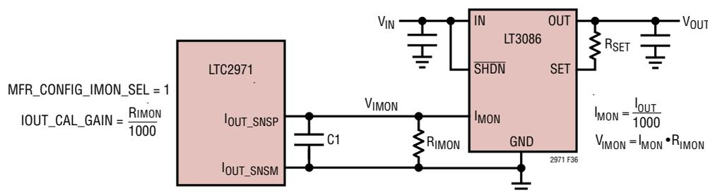
Figure 36. IMON Current Sensing
