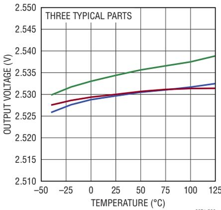
**V<sub>DD33</sub> Regulator Output Voltage vs Temperature**
