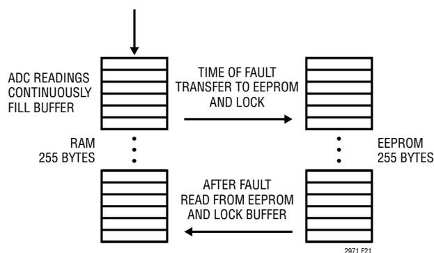
Figure 21. Fault Logging
