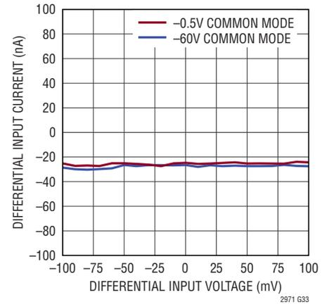
**+1.8V Channel Current Sense Differential Input Current vs Differential Input Voltage**
