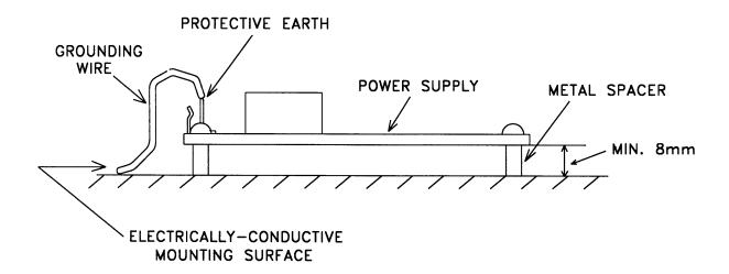
2. TO MEET SAFETY REQUIREMENTS, THE POWER SUPPLY TERMINALS MUST NOT BE USED DIRECTLY AS THE EXTERNAL TERMINATIONS OF ANY EQUIPMENT.
