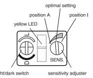
For optimal setting, now turn the sensitivity adjuster to the middle position between the positions A and B.
